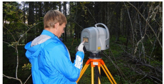
Figure 1. This terrestrial laser scanner from Trimble is used by SLU in forest inventory research projects. It produces one million millimeter-accurate 3D coordinates per second from points in the terrain that the laser beams are reflected from.
