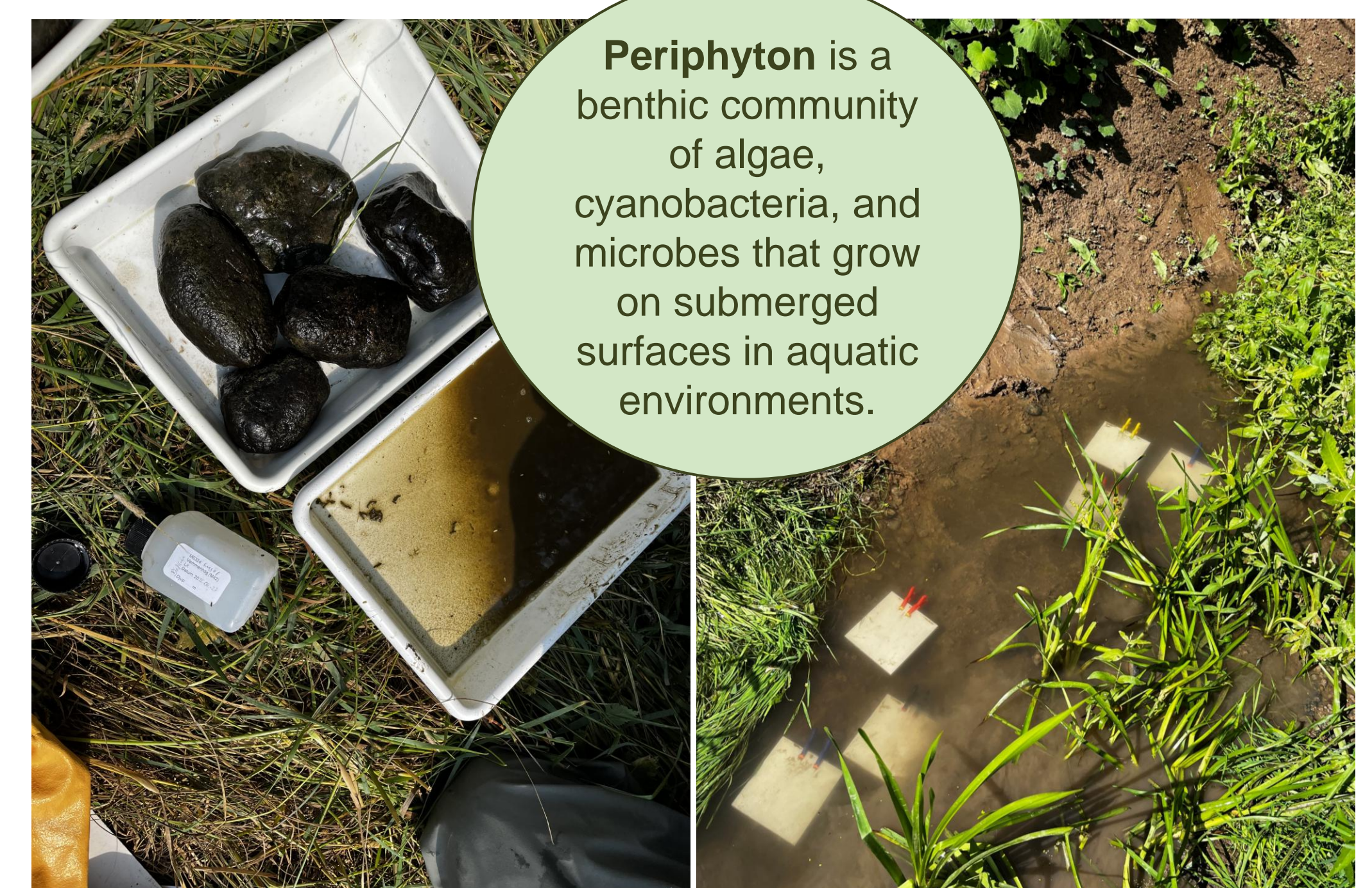
Standardized method to collect periphyton from natural substrate (SS-EN 13946:2014).
